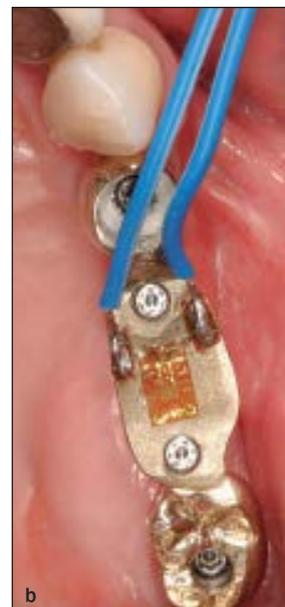
**Fig 1b** (right) Situation of an intraorally bonded FDP fixed in the oral cavity of a patient for in vivo strain measurements at the pontic site.
