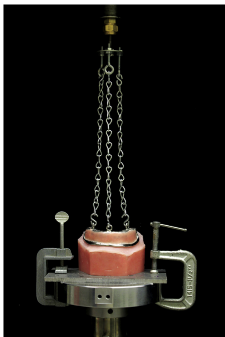
3 Experimental test model attached to universal testing machine base with clamps; washer, eye bolts, and pivoting joint assembly allowed for adjustment of chain slack and for correction of pivoting throughout experimentation.
