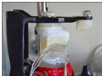
Fig 5 Image of loading. A vertical load of 98 N was applied with a loading apparatus to the lower dentition through the articulator placed upside down.
