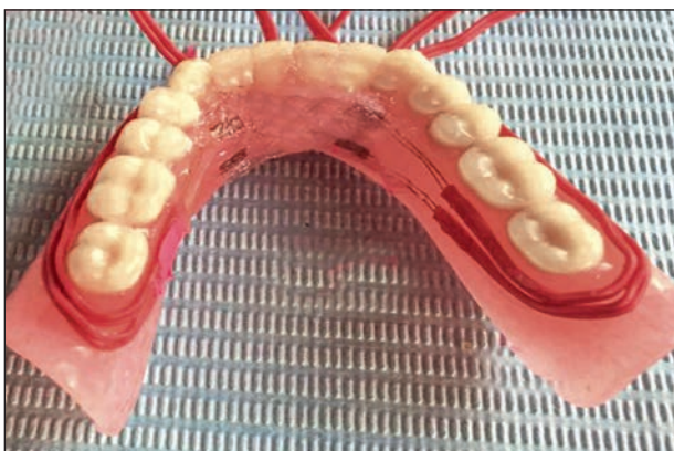
Fig 6 Isolated strain gauges attached to the polished surface of the denture.
