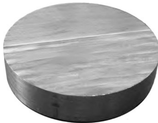
Figure 8 Titanium alloy blank prior to placement into milling machine for milling a CAD/CAM implant framework (Biomet 3i, Palm Beach Gardens, FL).
