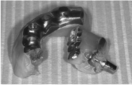
Figure 5 Laboratory image of a fractured fixed, implant-retained mandibular prosthesis. This prosthesis fractured through the distal cylinder on the patient's right side. The fracture also included the occlusal portion of the implant. The exact cause of this failure was unknown, although the vertical height of the framework appeared to be approximately 3+ mm.
